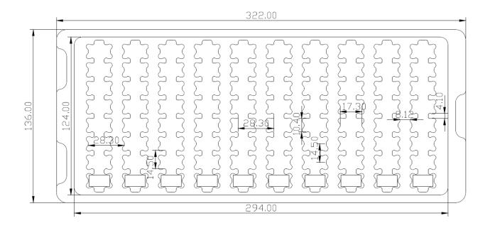
The tray is designed for direct use on a SMT automatic machine.
